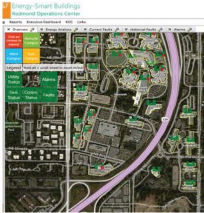
FIGURE 1: The Redmond Operation Dashboard used to monitor Microsoft's headquarter campus consisting of 125 buildings and 58,000 housed personnel.
